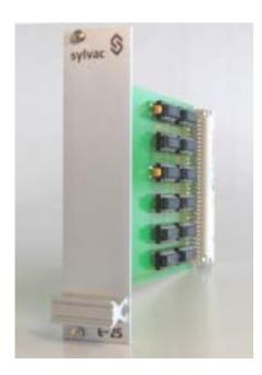
This board allows to extend the inputs of the converter board from 32 to 104.
