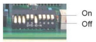
The switches 4 to 10 allow the selection of the probe type (P5, P10, P25 or P50) and the range of the output voltage :
