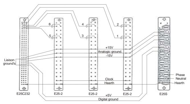
The digital and the analog mass is linked at one point of the E25C232 converter board input.
