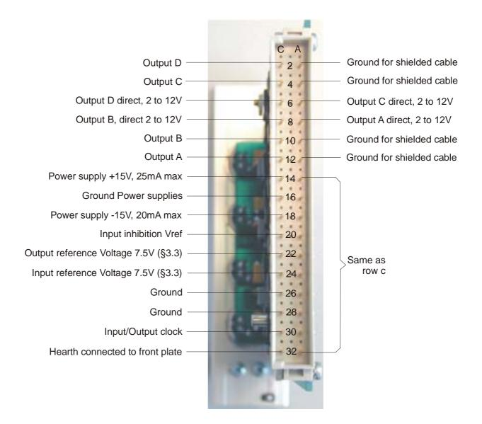
Output probe A (contact 12c) : from 0V probe in extended position to +10V, probe in compressed position Output probe B (contact 10c) : from 0V probe in extended position to +10V, probe in compressed position Output probe C (contact 4c) : from 0V probe in extended position to +10V, probe in compressed position Output probe D (contact 2c) : from 0V probe in extended position to +10V, probe in compressed position
